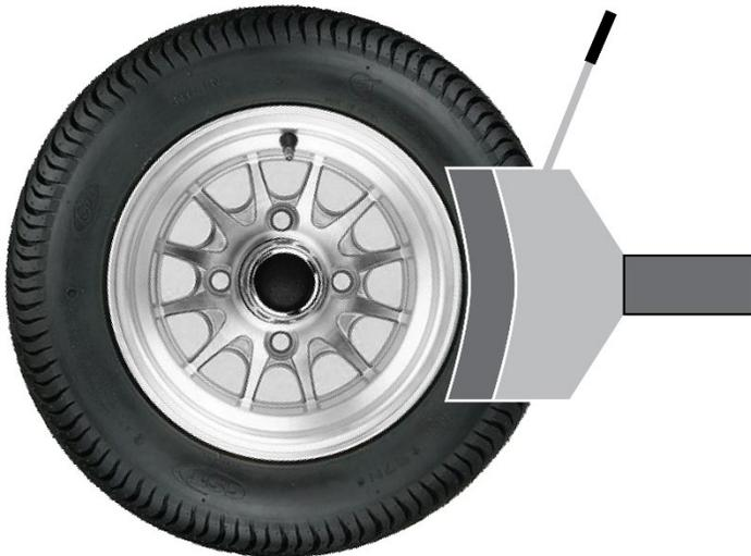
8. Move the Blade so that it is on the side of the Tire, very close to, **but not touching**, the Rim.
