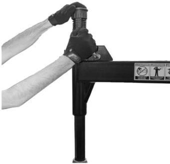
Pull the locking handle to lock the Vertical Shaft into position. As the Shaft is locked, the Mount/Demount Head will move upward approximately 1/8 in. (3.175 mm) and backward 1/8 in. (3.175 mm) from the rim's edge, thus providing operating clearance.
