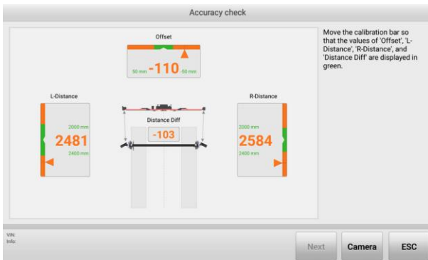
Figure 10-40 Accuracy Check Screen (Using a Calibration Bar) 2
