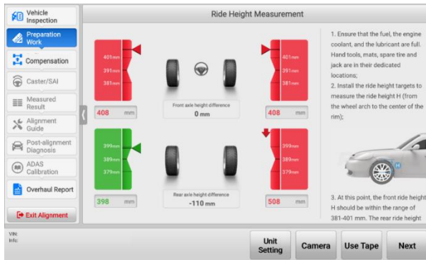
Figure 5-34 Measure Ride Height with Ride Height Target
