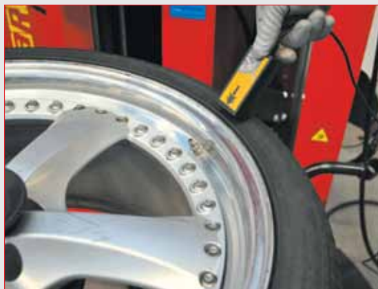
instrument for capturing sensor parameters
