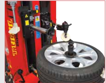
Automatic tool positioning for manual cycle
